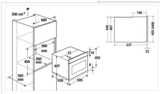
Minimum 200mm<sup>2</sup> at the back must be provided for ventilation.
